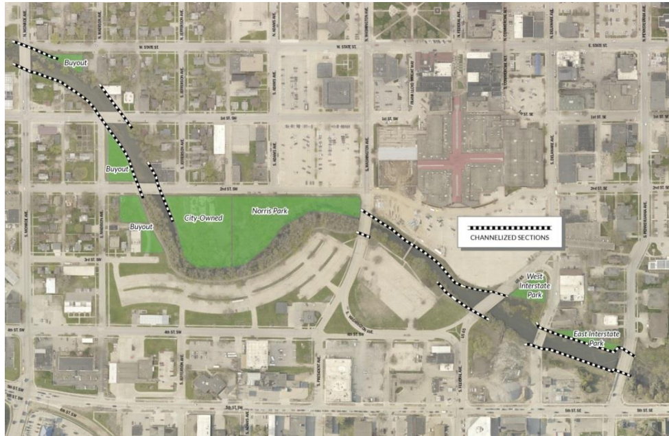
Sections of Willow Creek with channelized concrete floodwalls, and locations of open spaces and parks along the corridor
